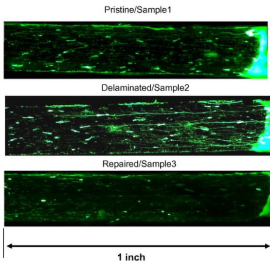
Fig. 7: Microscopy images of fluorescent dye on the transverse cross-section surface of pristine, delaminated, and repaired BMI–cf specimens.
