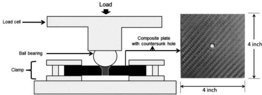
Fig. 2: The hole plate shear (HPS) test setup. HPS specimen is shown on the right.
