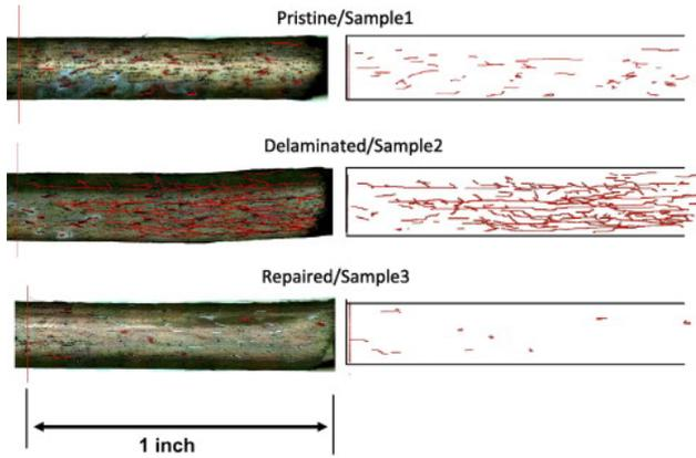
Fig. 8: Microscopy images of the transverse cross-section view of BMI–cf specimens with traces of cracks on the left side and a skeletonization of the crack lengths on the right side.
