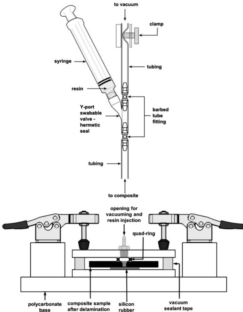
Fig. 4: Setup used for the injection repair process. The tubing from the vacuum pump and resin syringe are connected to the opening of the specimen chamber.
