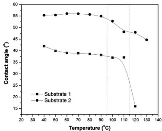
Fig. 5: Influence of temperature on the contact angle of BECy on BMI–cf substrate. The characteristic temperature range desired for repair is indicated between the dotted lines.
