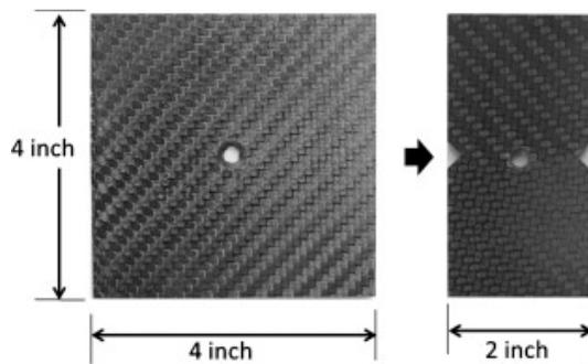
Fig. 3: Specimen modification for compression after impact test (CAI). Notches were added on both sides of the HPS specimen to prepare specimens similar like DENT specimen for post delamination compression tests.
