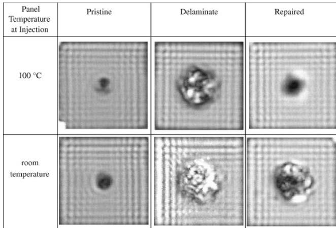
Fig. 6: C-scan images of pristine, delaminated, and repaired specimens repaired at room temperature and at 100 °C.
