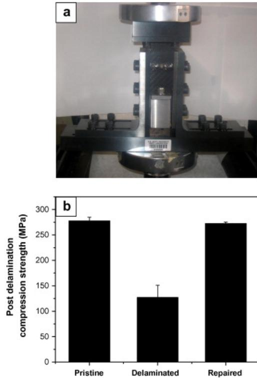
Fig. 10: Post delamination compression stress of pristine, delaminated, and repaired specimens. (a) Experimental setup for post delamination compression tests with double-edge-notched-tensile (DENT) specimen. (b) Maximum post delamination compression stress of pristine, delaminated, and repaired specimens.
