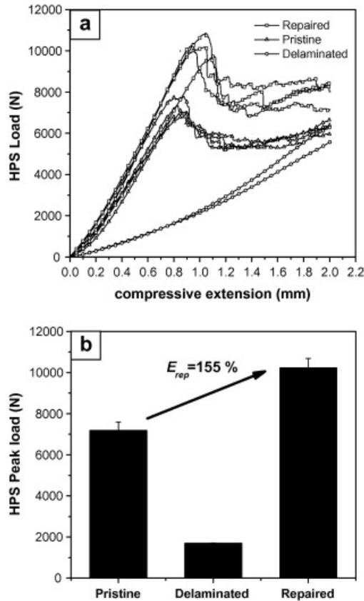
Fig. 9: HPS testing of pristine, delaminated, and repaired specimens. (a) Load–compressive extension curves for the investigated HPS specimens. (b) Maximum HPS load from load–compressive extension curves.
