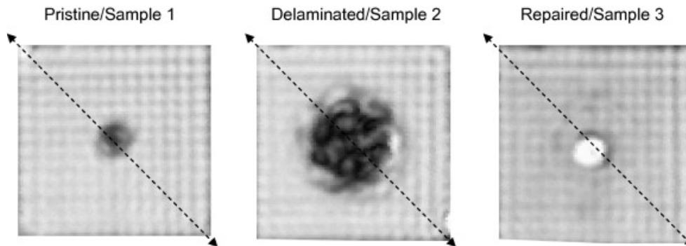
Fig. 1: C-scan images of pristine, delaminated, and repaired specimens used for fluorescent dye penetration and optical microscopy investigations.
