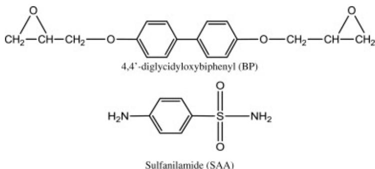
Fig. 1: Chemical structures of the epoxy monomer and the curing agent.
