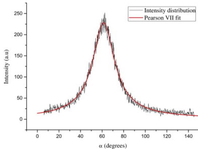
Fig. 7: Intensity distribution evaluated by integration through the inner diffraction ring of LCERs with a step size of 0.02 deg. The red line is the Pearson VII fit of the experimental data. (For interpretation of the references to color in this figure legend, the reader is referred to the web version of this article.)
