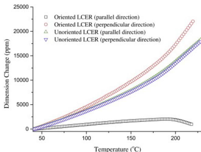
Fig. 10: Dimension change of oriented and unoriented LCERs upon heating.
