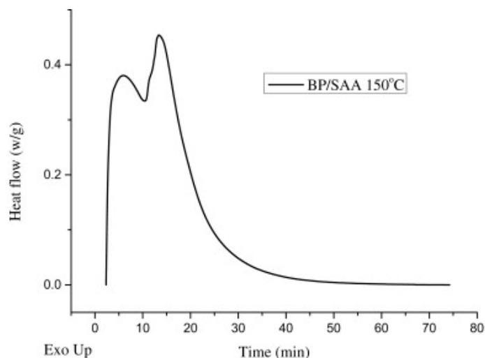
Fig. 2: Isothermal DSC curve showing the exothermic cure of BP with SAA at 150 °C.
