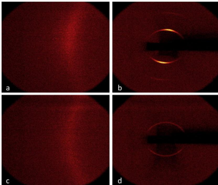
Fig. 5: XRD patterns of oriented LCERs and unoriented LCERs. (a), (b) Oriented LCERs at  $2\theta = 34^\circ, 0^\circ$ . (c), (d) Unoriented LCERs at  $2\theta = 34^\circ, 0^\circ$ .
