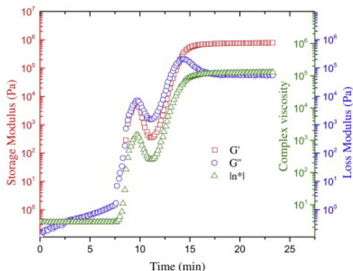
Fig. 3: Evolution of the complex viscosity, storage ( $G'$ ), and loss ( $G''$ ) moduli as a function of the reaction time at 150 °C (frequency = 1 Hz).
