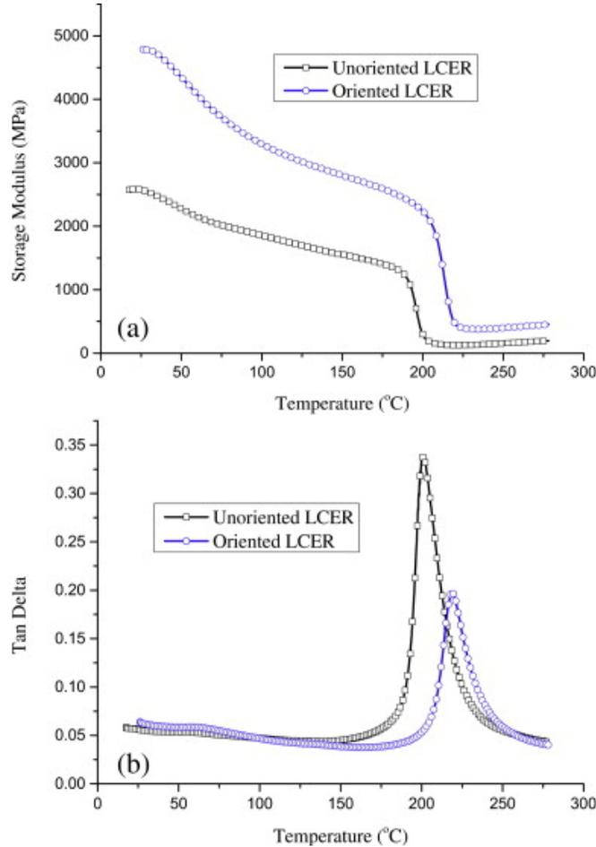
Fig. 9: Dynamic mechanical properties of oriented and unoriented LCERs. (a) Oriented LCER; (b) Unoriented LCER.
