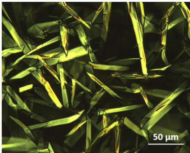
Fig. 4: POM image after 1 h of isothermal curing of BP with SAA at  $150^\circ\text{C}$ .
