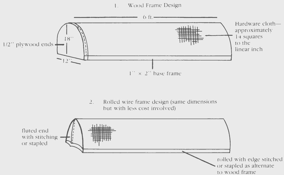
These designs are suggestions, and modification will suffice if it adequately keeps out flies. Whatever design is chosen, secure edges into soil, and if wind could be a problem, then secure with stakes and wire. For storage, either disassemble and hang on garage wall, or make each subsequent cage a little shorter and stack like sawhorses.
