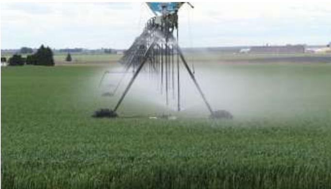
Figure 3. Madison's 15 psi low-hanging irrigation nozzles use just 7.5 gallons per minute. Photo: Darrell Kilgore.
