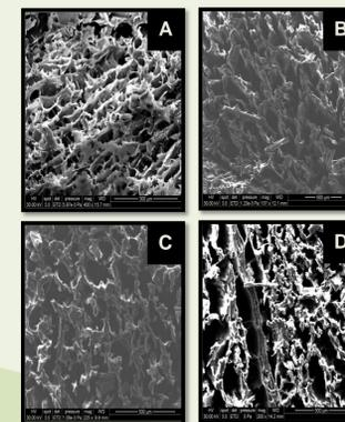
Figure 1. Scanning electron microscopy pictures of frozen salmon subjected state transitions during 4 weeks storage. (A) Salmon immediately after freezing, (B) Frozen salmon with  $T < T_g'$ , (C)  $T_g' < T < T_m'$ , (D) ( $T > T_m'$ ).
