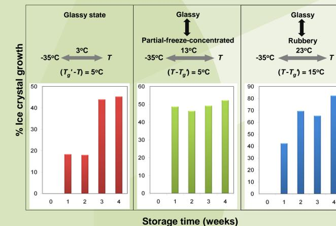
Figure 3. % growth in ice crystal size in frozen salmon subjected to fluctuations during one month storage of frozen salmon. Where  $T_g'$  = Glass transition temperature of maximally-freeze-concentrated matrix,  $T$  = Fluctuation temperature
