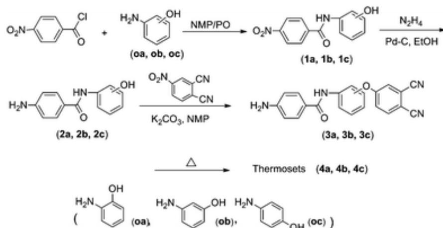
**Scheme 1** Synthesis and polymerization of **3a**, **3b** and **3c**.
