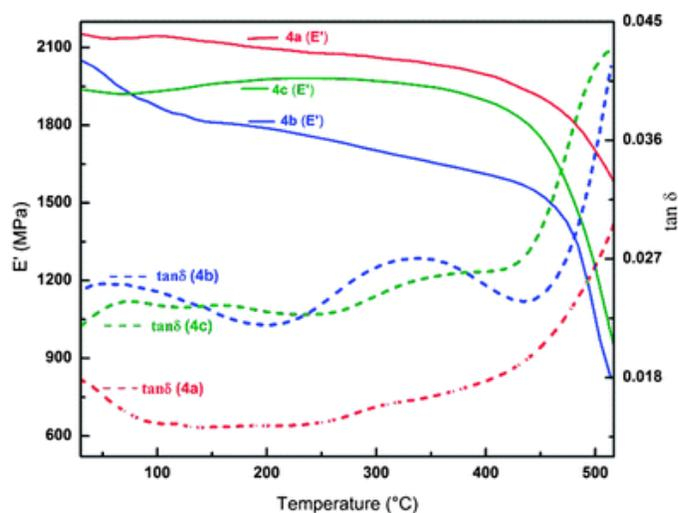
**Fig. 4** Storage moduli ( $E'$ ) and damping factors ( $\tan \delta$ ) of the polymers **4a**, **4b**, and **4c**.
