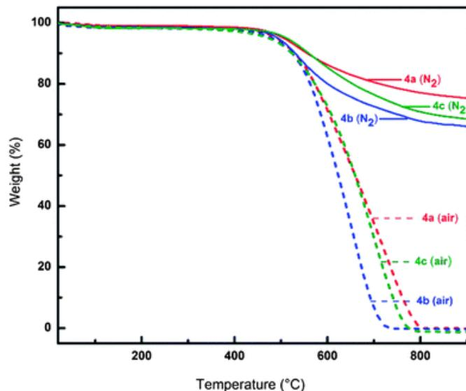
**Fig. 3** TGA plots for **4a**, **4b**, and **4c** in nitrogen and air atmospheres.
