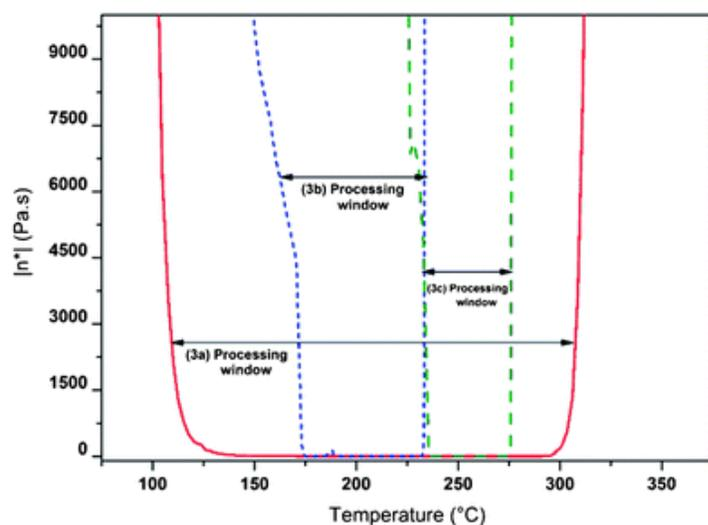
**Fig. 2** Complex viscosity ( $\eta^*$ ) of the monomers **3a**, **3b**, and **3c**.
