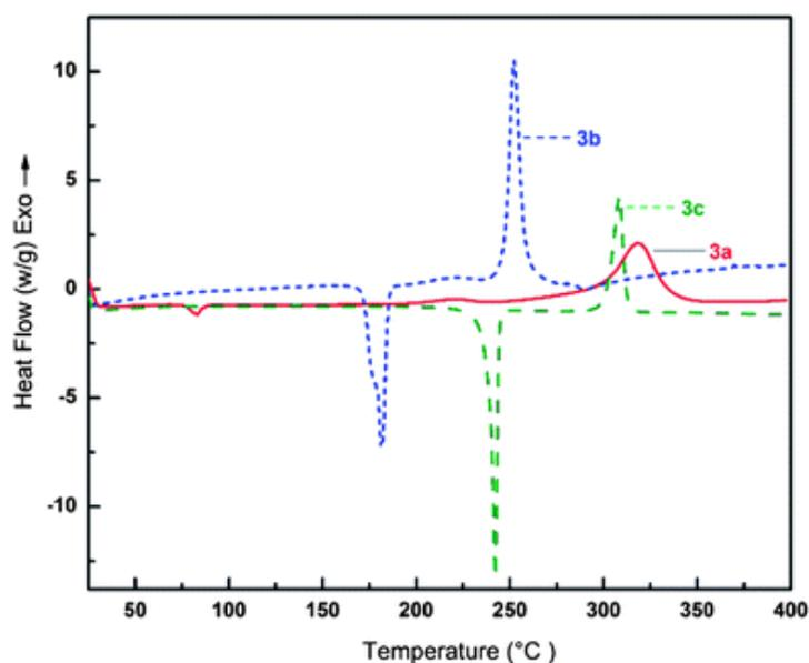
**Fig. 1** DSC curves of the monomers **3a**, **3b**, and **3c**.
