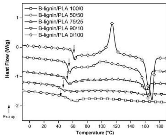
Fig. 3: Differential scanning calorimetry (DSC) curves for B-lignin/PLA blends.
