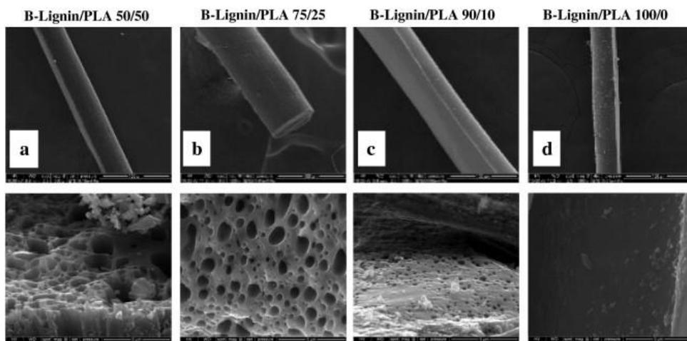
Fig. 6: SEM images of carbon fibers from B-lignin/PLA blends. Micrographs showing overall structure of the fiber (top) and cross-section images of the fibers (bottom); B-lignin/PLA (w/w): (a) 50/50; (b) 75/25; (c) 90/10; (d) 100/0.
