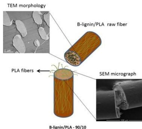
Fig. 2: Composite image showing the cross-section morphology and overall microstructure of B-lignin/PLA 90/10 blend fibers with PLA-rich phases self-assembled as micro fibers inside the bulk fiber.
