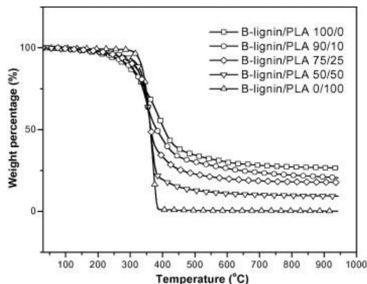
Fig. 4: Thermogravimetric analysis (TGA) weight loss curves of B-lignin/PLA blends.
