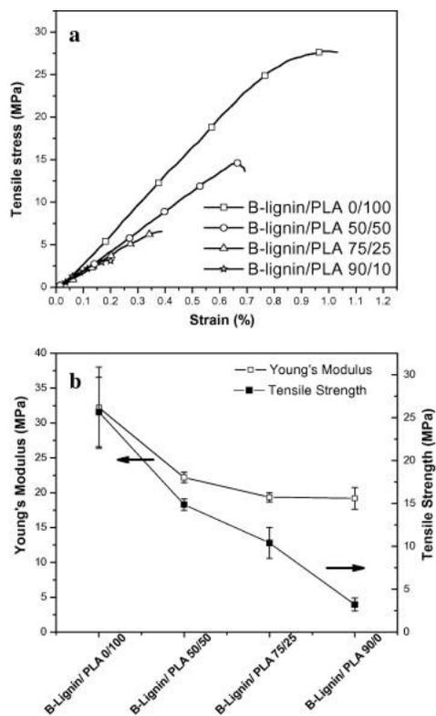
Fig. 5: Tensile mechanical properties of B-lignin/PLA precursor fibers. (a) Influences of blend composition on the stress–strain behavior of the fibers. (b) Young’s modulus and tensile strain at break determined by tensile test data.
