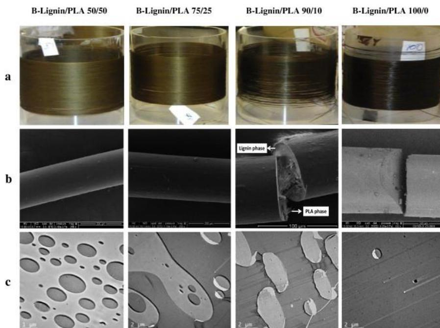
Fig. 1: Continuously spooled fibers of B-lignin/PLA blends (concentration of B-lignin increasing from left to right). (a) Fibers spooled on Pyrex glass mandrels. (b) SEM images of blend fibers showing overall structure of fibers. (c) Morphology of phase separation from cross section surface of individual blend fibers observed using TEM.
