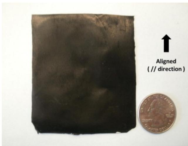
Fig 2: Optical image of dried BP sheet formed under a shear rate of  $1000 \text{ s}^{-1}$ .
