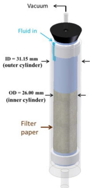
Fig 1: Schematic of modified Taylor–Couette system used to simultaneously shear and filter MWCNT dispersions. (A colour version of this figure can be viewed online.)
