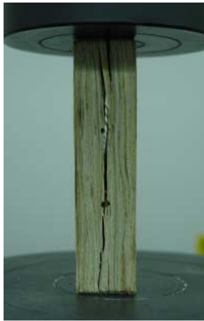
Figure 3: Tension perpendicular compression failure
