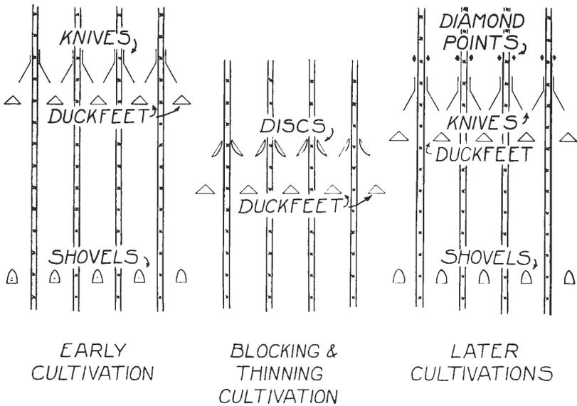
Fig. 4.—An alternate diagrammatic arrangement of cultivating and ditching tools.
