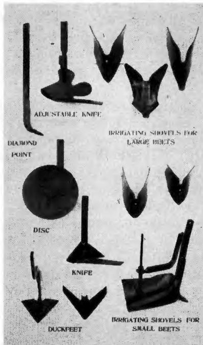
Fig. 2.—Types of cultivating and irrigating equipment for sugar beets.
