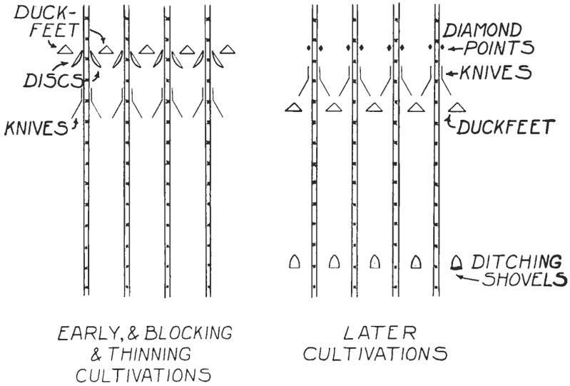
Fig. 3.—Diagrammatic arrangement of cultivating and ditching tools. This arrangement is preferred.
